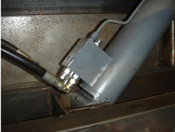
This photo **A**, shows a counterbalance valve which is pad mounted directly to the hydraulic cylinder. This too has no means integrated to identify and safely vent the isolated fluid. Making modifications to integrate test/bleed points requires engineering and may also include recommendations and acceptance by the equipment manufacturer. There would be a shift in liability and warranty if not done by the manufacturer when done by a modifier/integrator.
