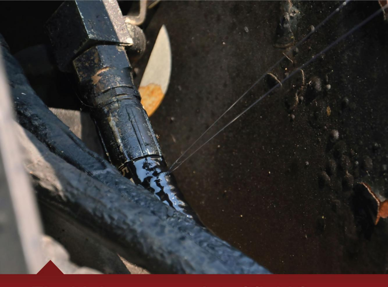
The high pressure jet of fluid from a pinhole rupture is extremely dangerous. Contact would cause a fluid injection injury which could lead to amputation.
